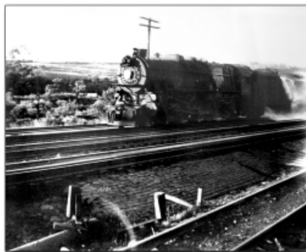
This 1943 picture of a passenger train going west bound at Wilmore, shows the train taking on water from the water pans. When the tender tank was full, it overflowed, as shown in the picture. A fireman then raised the scoop and the train kept going. submitted by Mark Blaisdell
